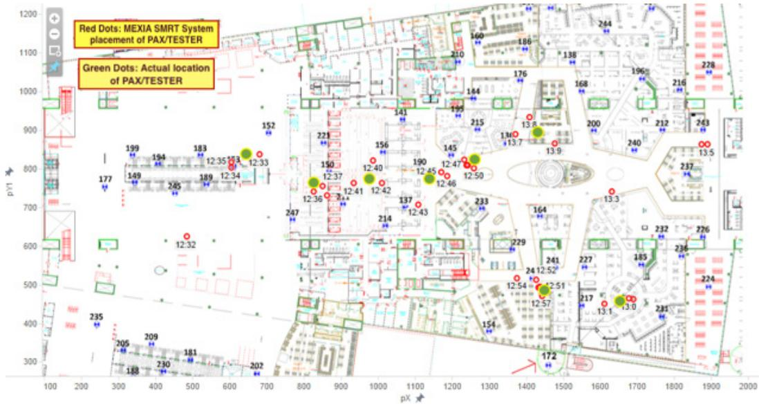
Test results of a blind walkaround. Green dots show locations identified by client as to where they were and when. Red Dots show where MEXIA SMRT Sensor locates them to demonstrate high level of accuracy (most results are within 2 meters).
